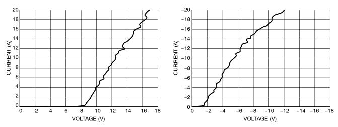
Figure 7. Positive and Negative TLP Waveforms
