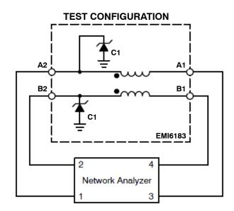
Normal (Differential) Mode Figure 3. Normal (Differential) Mode Test Configuration
